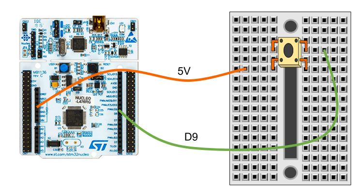
The switch needs to straddle the two sides of the breadboard
