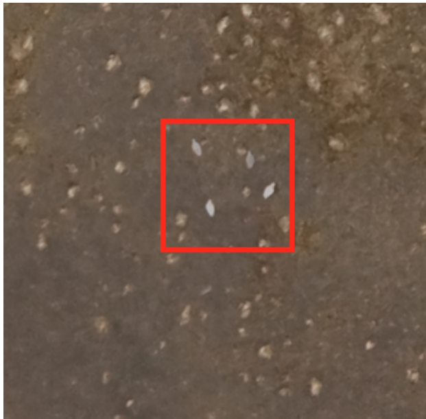
Fig. 7. Example of phantom objects created by the mosaicing process
